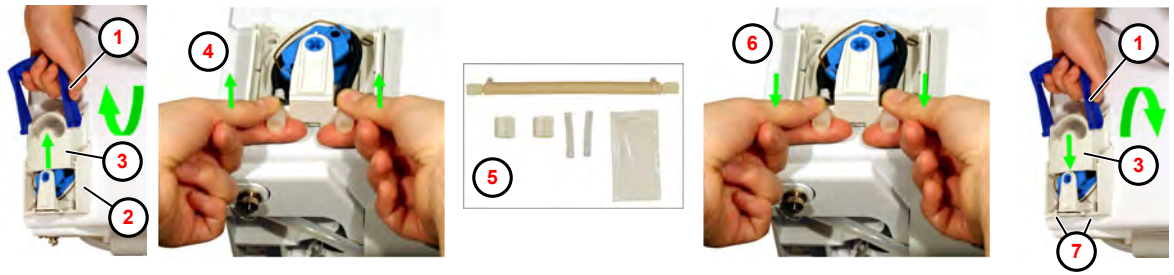
Fig. 22: Replacing the peristaltic hose
