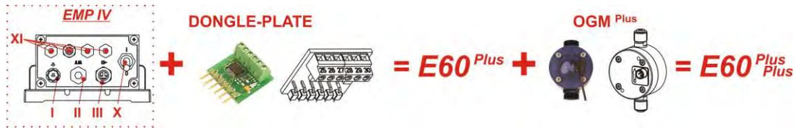
If an OGM Plus is connected, when the metering controller function is activated, the dosage quantity measured by the OGM is compared with a pre-defined dosage quantity target value. If there is a discrepancy between the values, the metering frequency of the pump is automatically increased or decreased.
