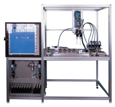
Fully automatic application of oil or adhesives with multifunctional equipment control
