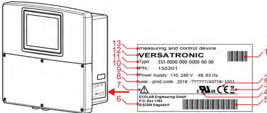
Fig. 1: Nameplate on device housing
