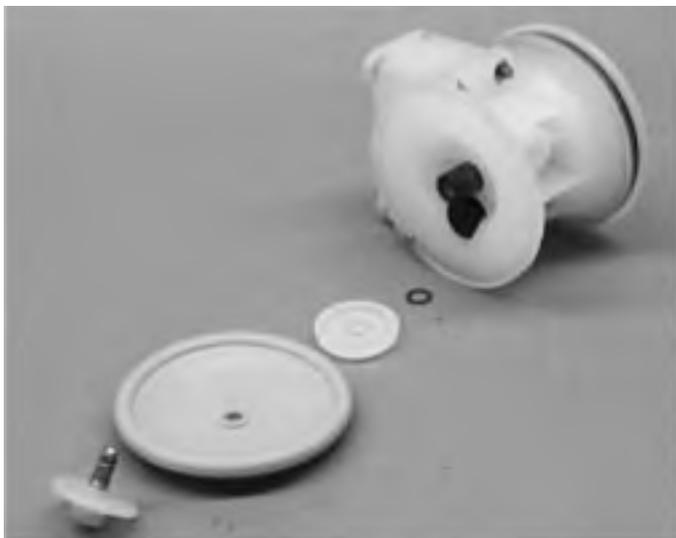
Elastomere/TPE Membran Konfiguration
