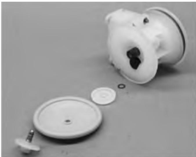
Elastomere/TPE Membran Konfiguration
