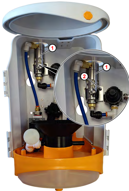
Fig. 16: Loosen the system separator
