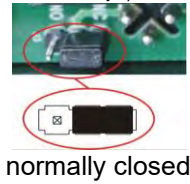
Fig. 7.27 normally closed contact
