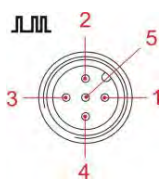
Fig. 7.16 Connector assignments of Slot I (3-terminal),
