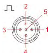
Fig. 8.9 Connector assignments of Slot VIII (5-terminal), input for pulse, standard signal input and metering lock
