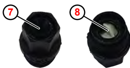
Fig. 15: Clean RTU Spray Nozzle_30
