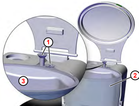
Fig. 10: Loosen the product cylinder
