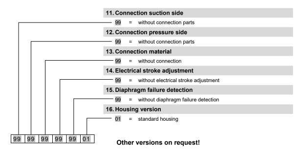
Example of a complete pump code of a standard pump:
