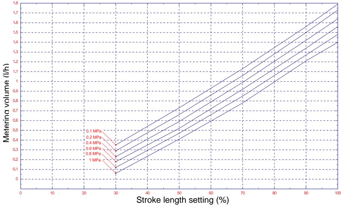
Fig. 14.9 Delivery capacity type V3014 / 1 MPa (10 bar)
