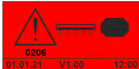
Fig. 26: Error code 206 (SMARTPOWER™ rinse aid)
