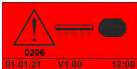
Fig. 10: Error code 206 (SMARTPOWER™ rinse aid)
