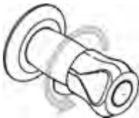
Fig. 11: Valve: Open water inlet
