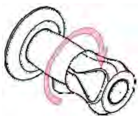
Fig. 20: Valve: Closing the water supply
