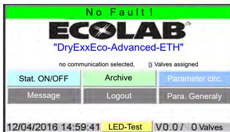
⇒ After successful system start-up, the 'start screen' appears in the display of the control cabinet.
