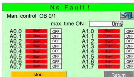
⇒ Screen 'Man. control OB 0/1' opens and shows the switching status of the digital outputs on the corresponding output interface.
