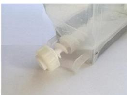
Empty the container completely. Then loosen the union nut by turning to the right (!) and pull the spindle out of the container. Carefully remove powder residues / lumps, then reinsert the spindle into the device and secure with the union nut. Turn union nut to the left (!) and tighten hand-tight.
