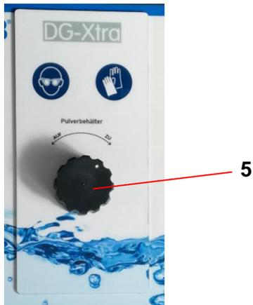
5 - Rotary knob for unlocking the powder container
