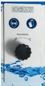
Unlock the rotary knob on the front by turning it to the left and carefully pull the powder container out of the device.
