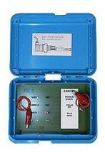
**Calibration box** for bleeding (conductive) with simulation resistances for the measurement ranges  $0 \dots 5, 0 \dots 50, 0 \dots 500 \mu \text{S/cm}$
