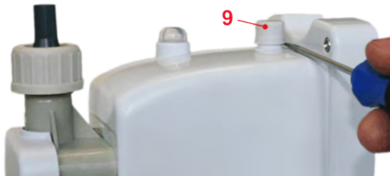
Fig. 8: Detaching the cover plug for speed adjustment at potentiometer
