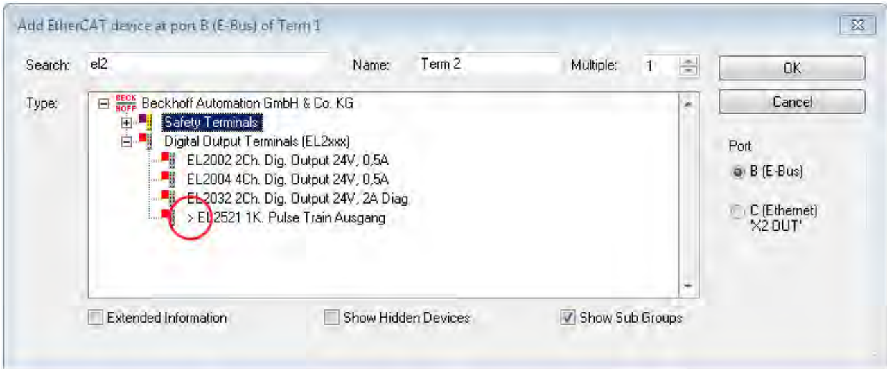
Fig. 89: Indication of an online recorded ESI of EL2521 as an example
