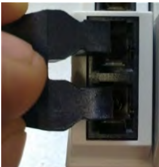
Figure: Blind plugs in unused sockets
