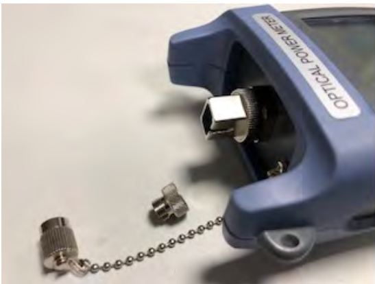
OPM with SC adapter screwed on
