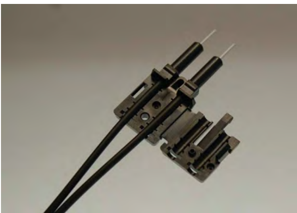
Fig. 55: Cable inserted in the connector
