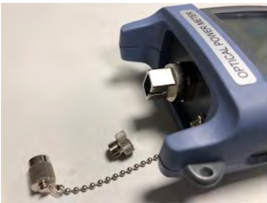
OPM with SC adapter screwed on
