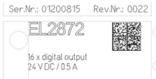
Fig. 3: EL2872 with revision 0022 and serial number 01200815
