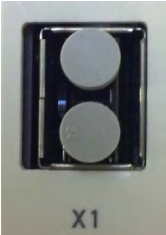
Figure: Blind plugs in unused sockets
