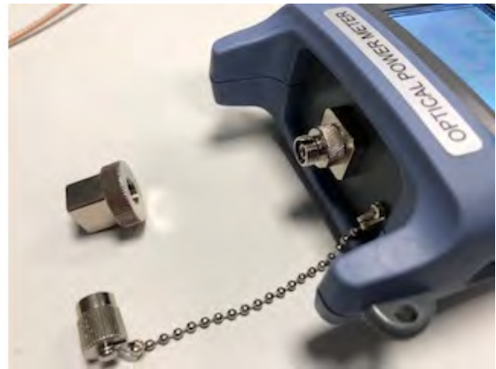
OPM with FC adapter screwed on
