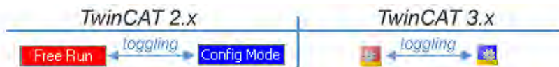
Fig. 129: Displaying of “Free Run” and “Config Mode” toggling right below in the status bar
