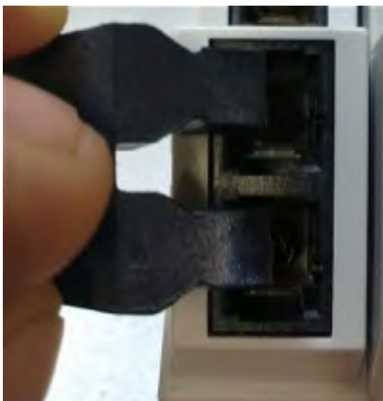
Figure: Blind plugs in unused sockets
