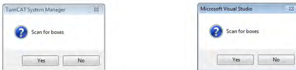
Fig. 109: Scan query after automatic creation of an EtherCAT device (left: TwinCAT 2; right: TwinCAT 3)
