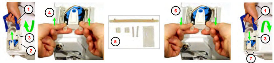
Fig. 23: Replacing the peristaltic hose
